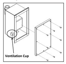
2. Reattach the cover and ensure that the opening of the ventilation cup is always facing the ground. If the position of the ventilation cup is changed, ensure to tighten it firmly.
